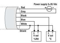
The instrument is equipped with a 7 wire + shield cable.
